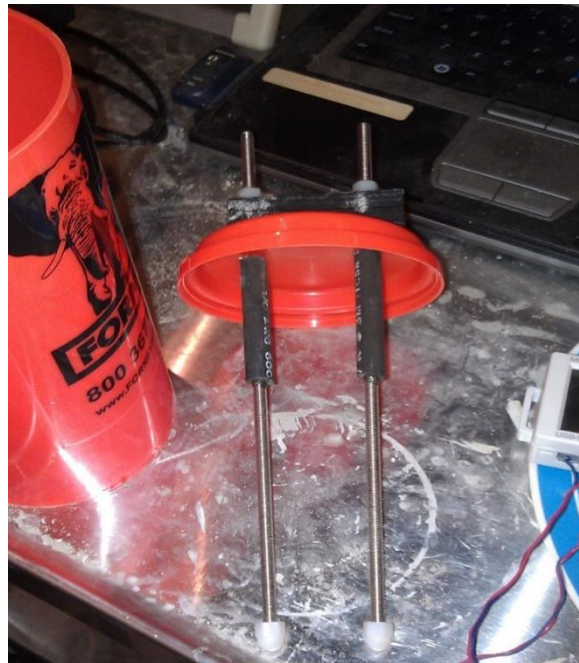
Figure 1. Twin steel screw rods for embedding in a cylinder of fresh concrete to measure its electrical resistance. The cap with holes is for a 100 mm by 200 mm concrete cylinder mold.
