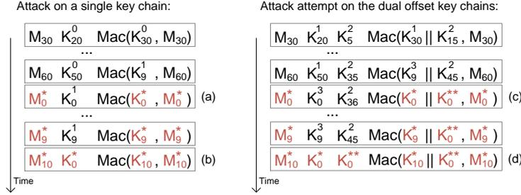
**Fig. 3.** Example of a man-in-the-middle attack on a single hash chain without commitment and on the Dual Offset Hash Chains mechanism.
