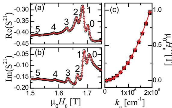
FIG. 2. (Color online) Measured  $S_{21}$  transmission parameter (black circles) at 20 GHz and the multi-peak-susceptibility fit (red line) for the (a) real part and (b) imaginary part obtained with the Ta(3)-Py(200)-Si<sub>3</sub>N<sub>4</sub>(3) sample. The first six modes are shown. (c) The exchange field  $H_n^{\text{ex}}$  (black squares) and exchange field fit, from Eqs. (9) and (10) (red crosses) for all 13 detected modes plotted as a function of the fitted wave numbers  $k_n$ .
