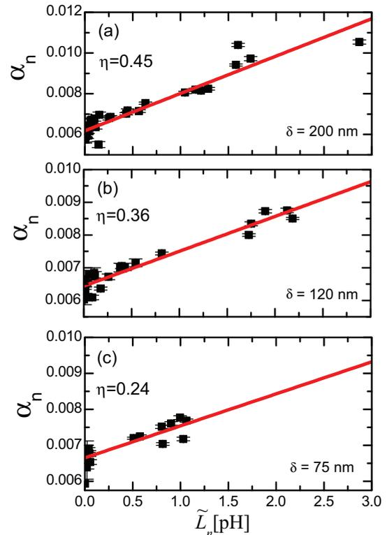
FIG. 5. (Color online) Dependence of damping  $\alpha$  on the normalized mode inductance  $\tilde{L}_n$  after correction for the eddy current damping  $\Delta\alpha_0$  of the fundamental mode, plotted for all sample configurations and different thicknesses: (a)  $\delta = 200 \text{ nm}$ , (b)  $\delta = 120 \text{ nm}$ , and (c)  $\delta = 75 \text{ nm}$ . The red lines are weighted linear fits to the data by use of Eq. (5), that describes the radiative component of the damping.
