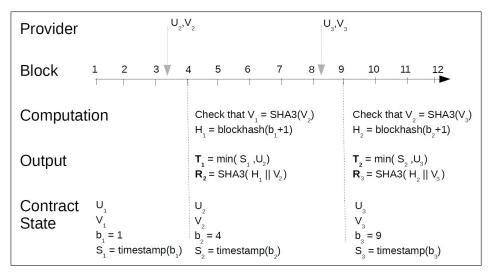
Fig. 1. The Single Producer Protocol
