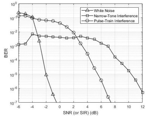
Fig. 2. BER of Turbo-coded OFDM, affected by white noise or interference.
